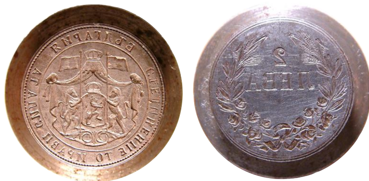
Fig. 3. Trial dies for Bulgarian 2 Leva piece.
