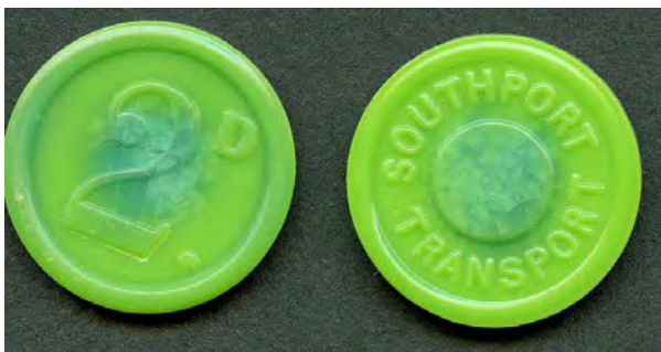
Fig. 2. Southport 2D green 715BH, two tokens stored in the same packet, showing typical cuboid cracking inside the token - not a surface effect. The acidity has also caused a colour change in the affected area.
