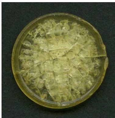
Fig. 4. Aberdeen 1/2D transparent 30AN typical advanced cuboid cracking
