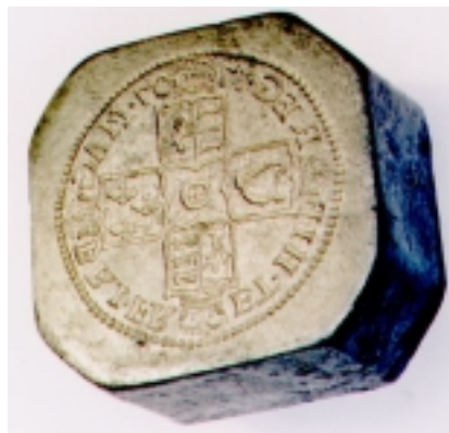
Figure 15. Contemporary counterfeiters' die for the reverse of a 1707 shilling
