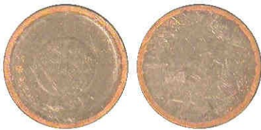
Fig.2: lead centre and copper rim
