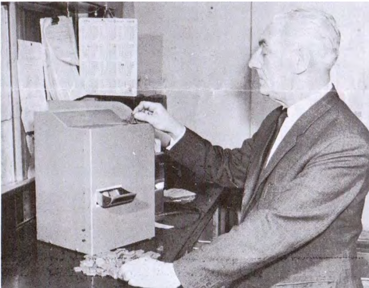
Senior booking Clerk Alf Hastings remagnetises tokens after use in the automatic machines at Stanmore
