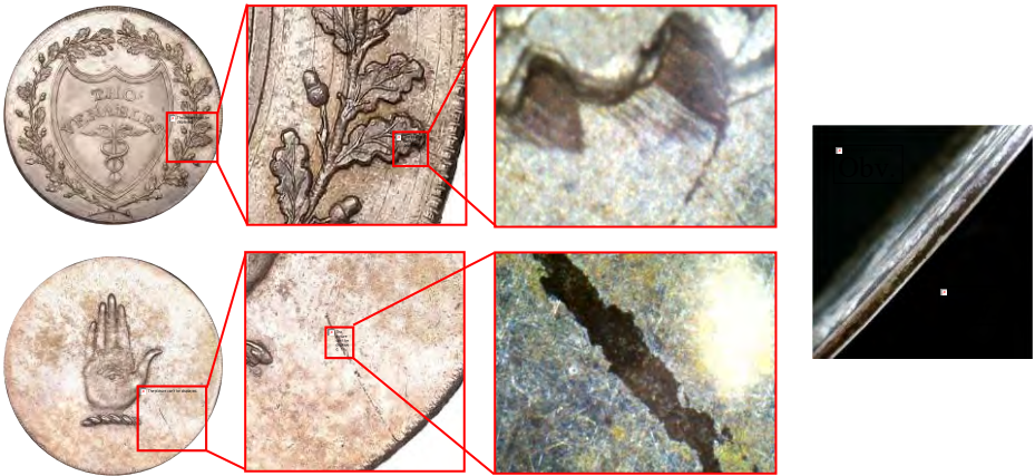
Fig. 1. Close-up and microscope image of obverse, reverse and edge revealing copper core of Thomas Venables' plain edge shilling token.
