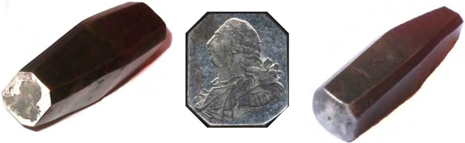
Fig. 1. Octagonal Punch, 51mm long, enlarged detail of face.
