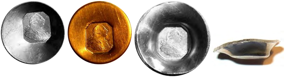
Fig. 3. Testing the punch in pewter, brass and a larger force in pewter (x1.5).
