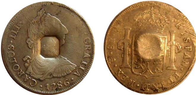
Fig. 4. Testing the punch on a 1786 Potosi Mint Dollar of Charles III.
